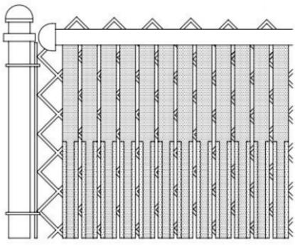
Insert the narrow end of each slat into the fence vertically.
