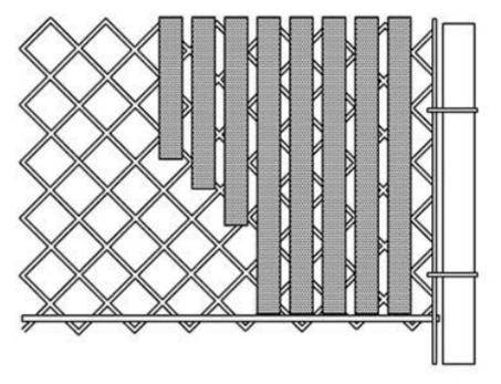
Insert the slats vertically into the fence from top to bottom.
