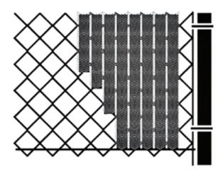
These Insert HedgeLink Slats vertically top to bottom, keeping the green needles facing up, while revolving the slat clockwise with your fingers for easier installation.
