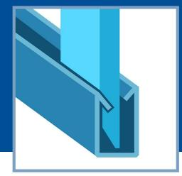
Insert the bottom locking channel horizontally into the bottom row of links on the chain link fence. Be sure the open side of the channel is facing up.
