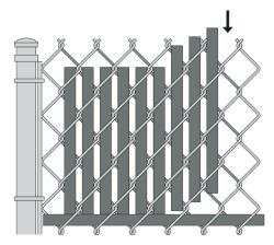
**Step 2.** Insert slats vertically with the beveled/notched end downward until slat engages and interlocks with the bottom channel.
