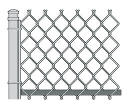
**Step 1.** Insert the bottom channel horizontally into the first diamond at the bottom of the fence with open side facing up.
