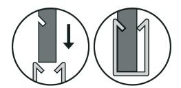
**Step 3.** Push the vertical slat into the horizontal channel until the locking catch snaps into the cutout notch.
