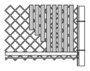
Insert rail horizontally in first full diamond at bottom of fence with open side facing up.
