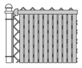
Push the vertical slat into the horizontal channel to lock in place.
